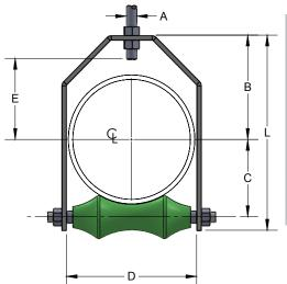
"E" Dimension includes exposed rod threads beyond bottom of hex nut. Exposed rod thread dimension is equal to the diameter of the rod used.
